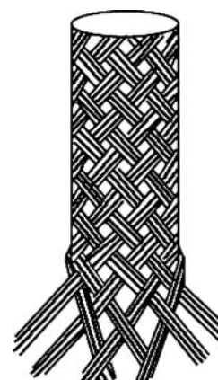
Figure 3 Schematic of a microbraided tubular construct.
