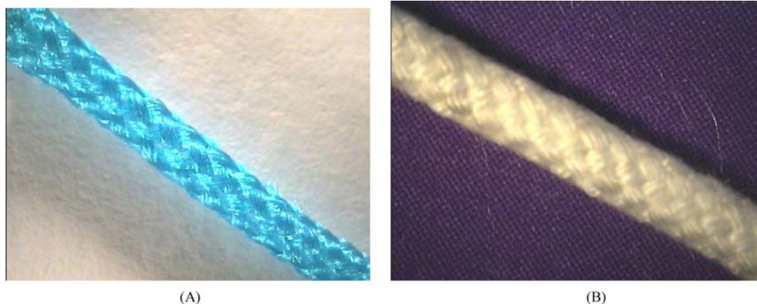
Figure 4 Macrograph of the tubular scaffold (A) PLGA (B) Chitosan.
